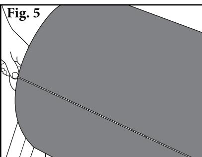
5. **After the first coat of adhesive has dried completely, mark a line across the pulley face using a chalk line or scribe, ensuring the line is parallel to the shaft's centerline and square to the edge of the pulley.**
