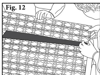
12. Follow Steps 6 through 10 to install the last 3-4 strips. The final piece of lagging (largest of final pieces) should drop into position. Check the fit of the last piece prior to applying the second coat of adhesive.
