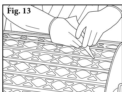
13. Fill any gaps between the lagging strips with rubber sealer. Also use the buffing wheel on trimmed edge of lagging and apply final coat of adhesive to seal the edge and joint area between lagging strips.
