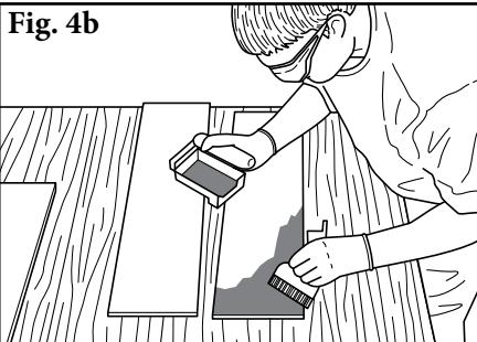
4. **Apply first coat of adhesive.** Thoroughly mix one can of adhesive and one activator at a time, immediately applying it to the pulley and strips of lagging. Be sure to apply adhesive to the edges of the lagging as well. This process should use half of the adhesive/activator required in the chart on Page 6. **Note: Allow to dry for a minimum of 25 minutes at 23°–25° C (73°–77° F). Temperature and humidity will affect dry time.**
