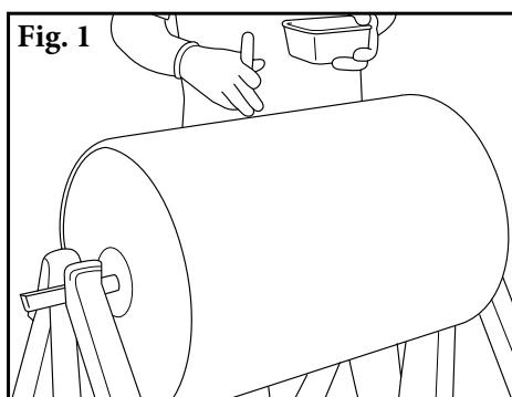
1. **Prepare the pulley by removing the old lagging, paint and primer.** Sand blast the entire pulley or use a grinder with 24 grit flap disc or paper disc. Use bench brush and non-oil-based metal solvent to clean remaining particles from the pulley surface. Paint the pulley surface, including the edges, with Flex-Lag Primer. Allow to dry completely – a minimum of 30 minutes.
