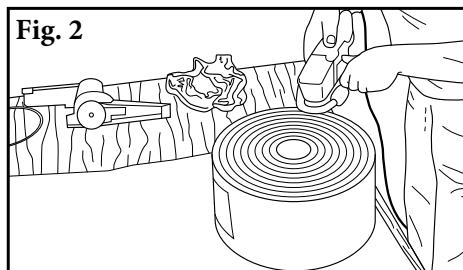
2. **Use a grinder with coarse dish wheel to buff the edges and bottom of the lagging.** Be careful not to smoke the rubber. Wipe with non-oil-based solvent to clean surface of any particles.
