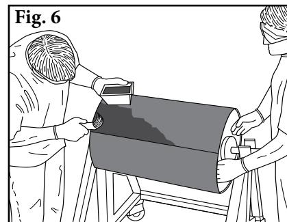
6. **Apply second coat of adhesive to the pulley.** Thoroughly mix one can of adhesive and activator at a time. From the perpendicular line, apply the second coat of adhesive to an area slightly greater than one strip of lagging.
